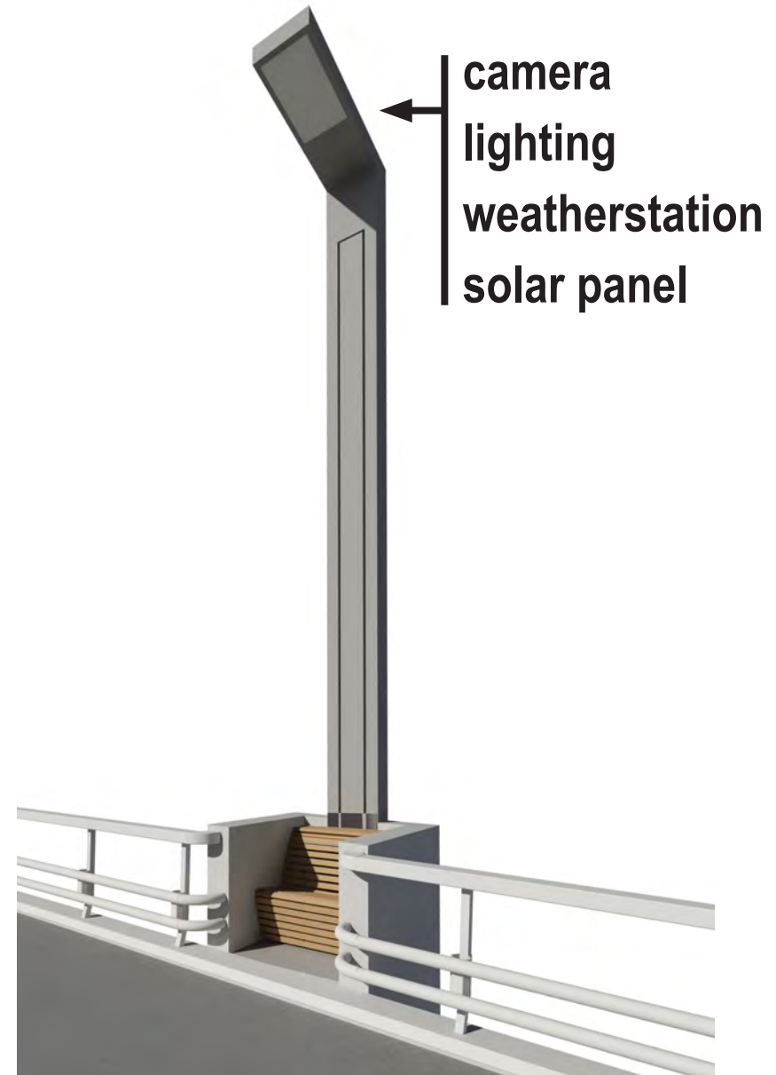
tiltable multi-functional mast for movable bridge
