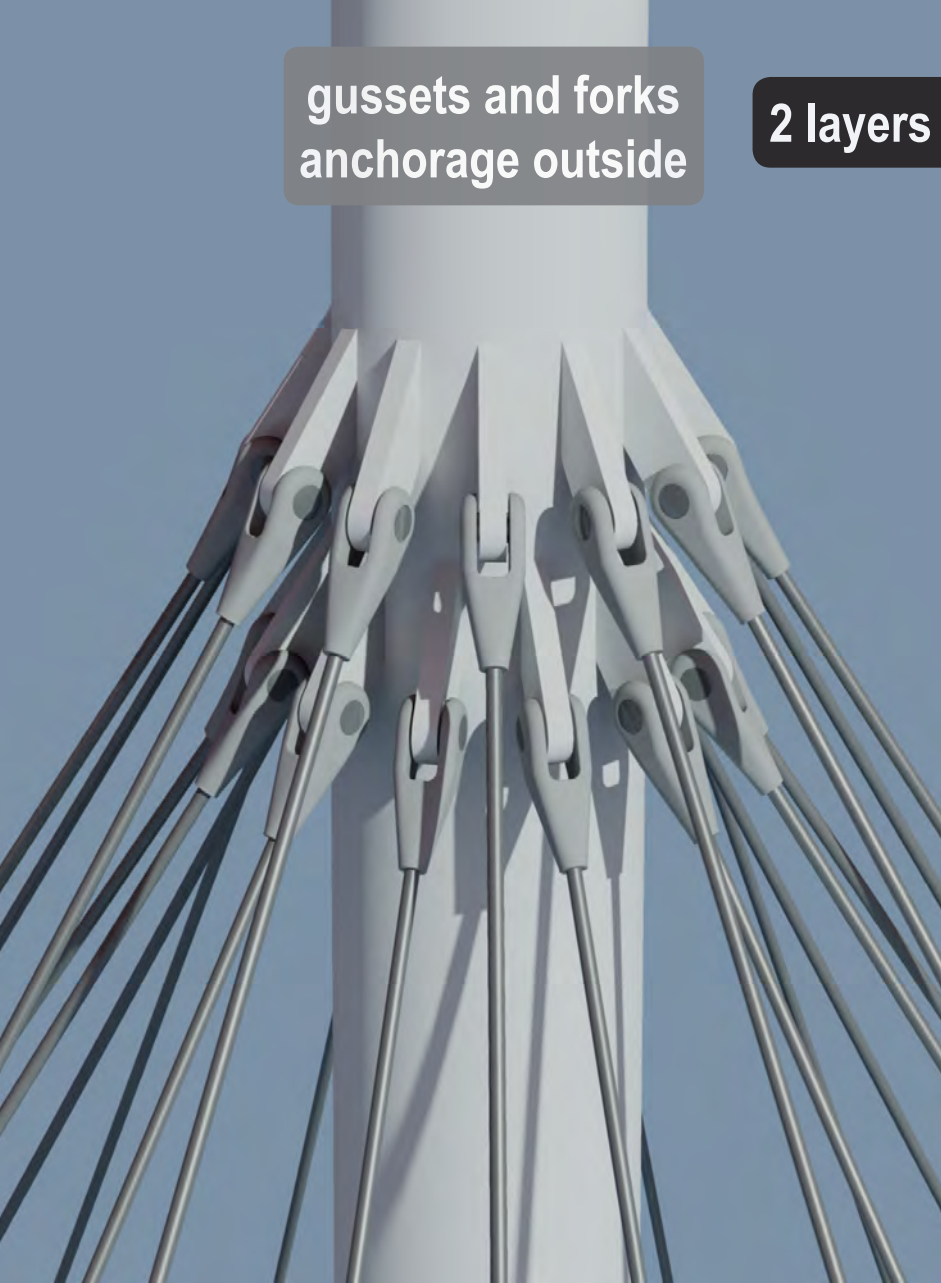
Design details Pylon Cable Anchorage
