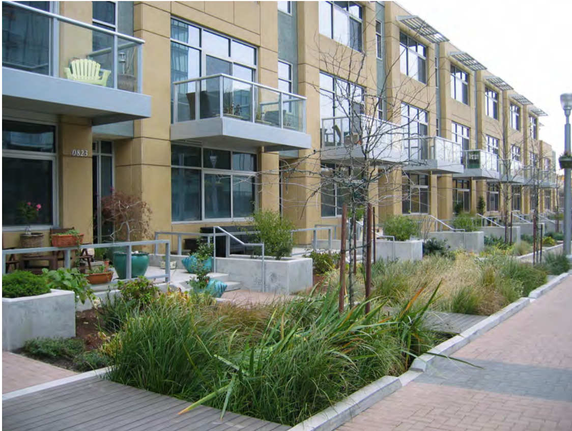
A Portland stoop frontage integrates usable space with stormwater gardens. Photo by Kelley Kahn
