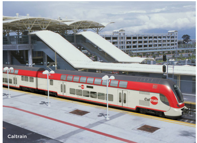
High-speed rail trains will use electric multiple units — train cars that receive power from overhead wires. Each car receives its own power, rather than having a single engine at the front or back of the trains.
