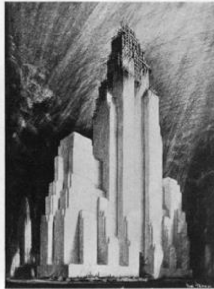
IV. THE MASS MODIFIED BY THE STEEL CONSTRUCTION. Its appearance after conforming the set-backs to the steel grillage and truncating the pinnacles to the highest floor level, which contains a practicable area. The mass is now ready for architectural articulation.
