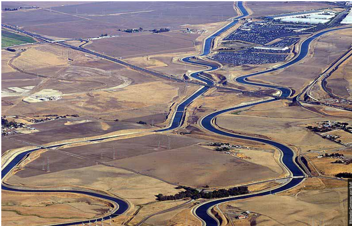
The California Aqueduct and Delta-Mendota Canal convey water through the delta to supply millions of water users in California.
