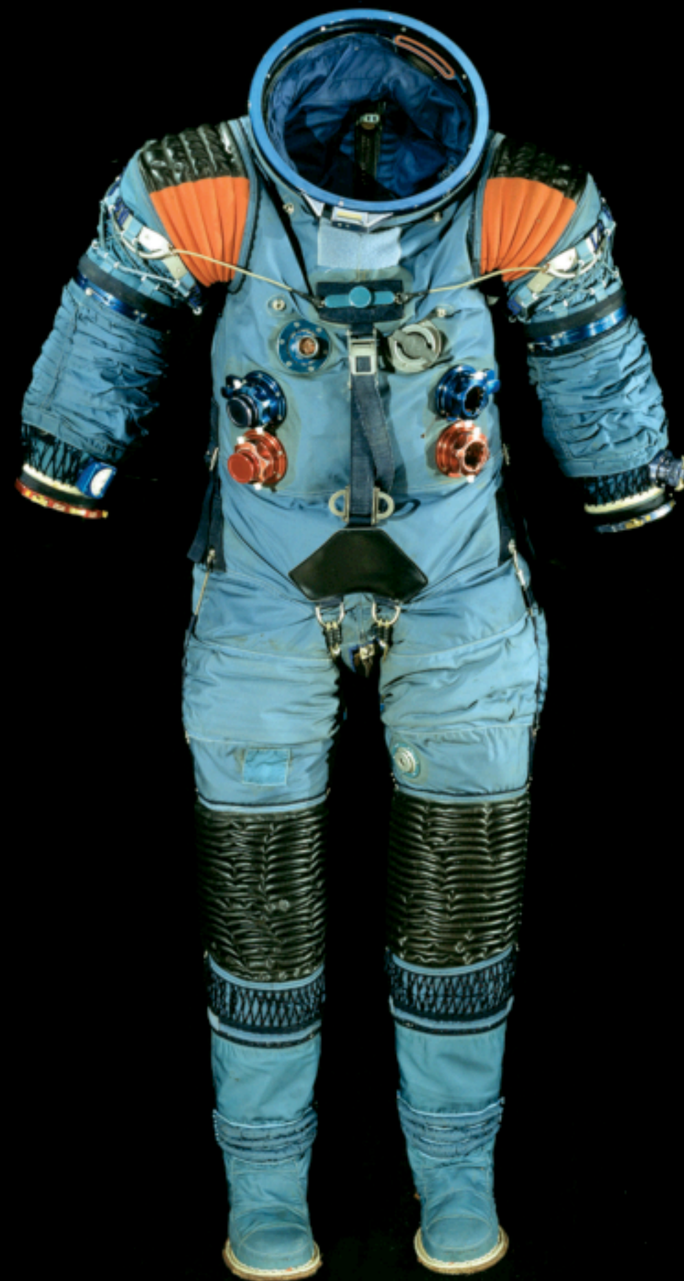
ILC A7L Spacesuit without white Thermal Micrometeoroid Garment (TMG). Photograph: Mark Avino, Smithsonian Institution
