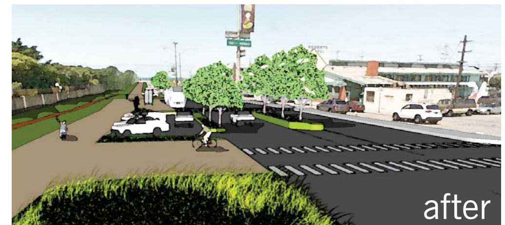
Figure V-4b: Proposed Sloat Blvd = Bike Lane + Pedestrian Walk + Diagonal Parking Pockets + 2 Driving Lanes + Planted Median + 2 Driving Lanes
