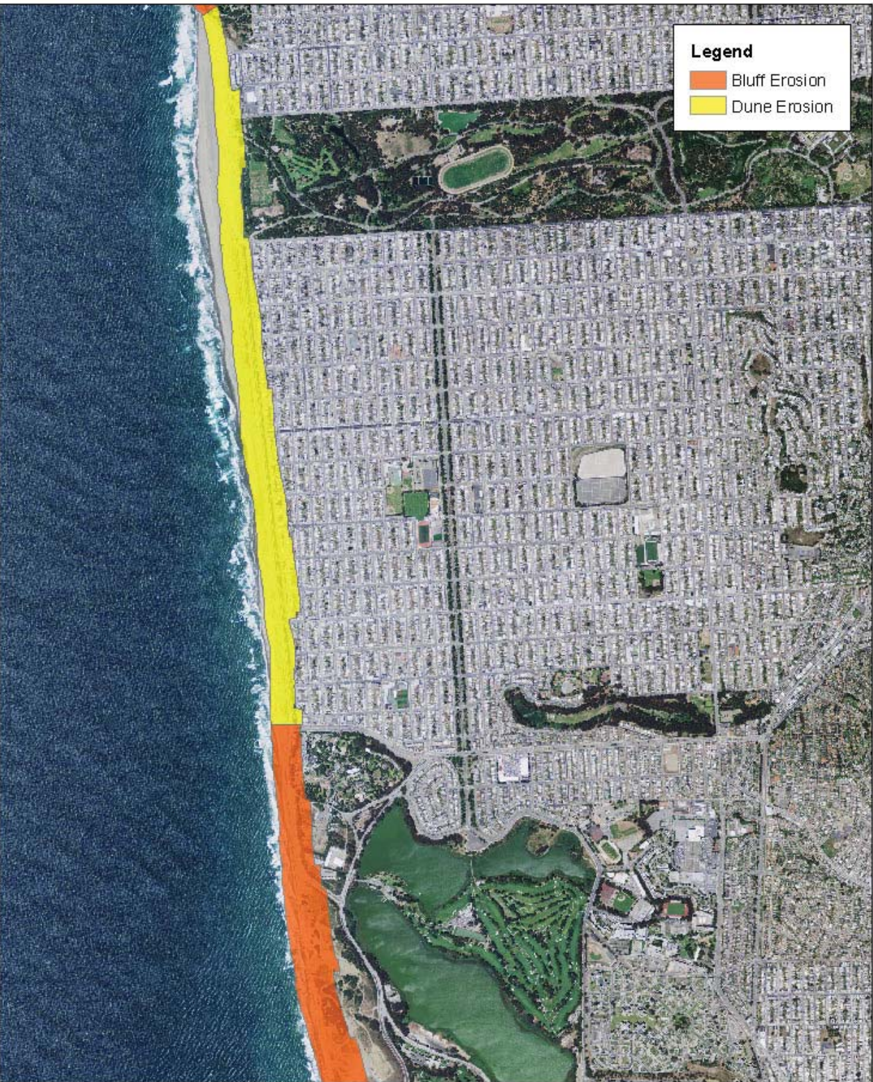
Figure 2. Bluff and dune erosion hazard zones predicted with 4.6 feet of sea level rise (after Pacific Institute 2009).
